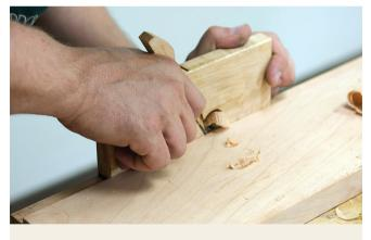
PLANE A RABBET. Set the blade slightly proud of the plane side so that it will clean the inside corner. Begin your planing stroke with the blade off the work. Keeping the plane level, lightly press down on the front of the plane and begin pushing it forward. As the blade bites into the wood, put more pressure on the center of the tool. At the end of the cut, shift pressure to the back of the plane so that the plane doesn't tip.
