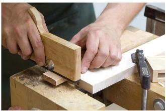
PLANING A TENON CHEEK is the same as planing a rabbet, but you may need to take several passes to work up to the shoulder. Remember to set the blade so that it's flush on the side that will make contact with the shoulder of the tenon you're tuning. Shave equal amounts off each tenon cheek for the perfect fit.
