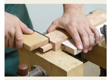
TO PLANE A SHOULDER, rest the side against the tenon's cheek and shave the end grain. Because you're cutting tough end grain, thin shavings are important. To avoid break-out, stop 1/8" to 1/4" from the corner and then complete the cut from the opposite side.
