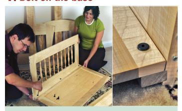
Position the base on the side cleats and insert the connector bolt and nut. Make sure that the ends are flush before tightening the three bolts.
