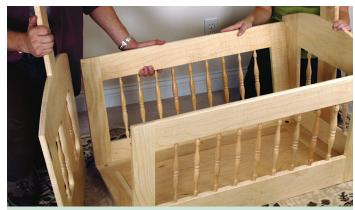
Note how the the keyhole hangers capture the four pairs of screw heads. Hold down the sides and pull up on each end to ensure that the joint is locked tight.
