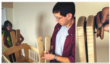
Arrange the uprights so that the keyhole hangers face in, then add the wood washers before inserting the dowels into the uprights. Now, screw the knobs onto the hanger bolts.
