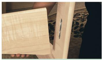
With one helper steadying the cradle, fit the screw heads into the hangers in both uprights and then tap the top of the stretcher to lock in the knock-down hardware.
