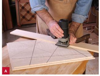
To rout the lines, set the bit to make a V-cut about \%" deep, and then run the router against a fence.
